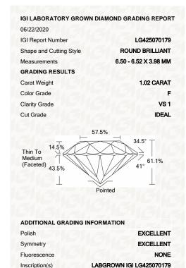
Comments: This Laboratory grown diamond was created by chemical vapor deposition process (CVD) Type IIa, No indications of post growth treatment.
